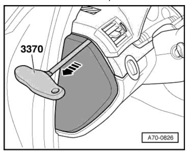
• Reach through opening - **arrow A** - above fuse panel and push out instrument cluster in direction of - **arrow B** -.
