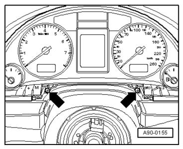
• Remove left instrument panel side cover - **arrow** - using hook (3370).
