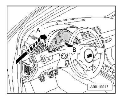
• Disengage lock on electrical connectors - arrow - and disconnect.
