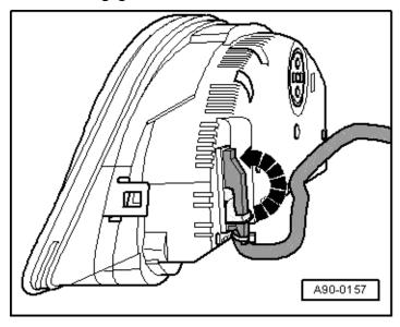
• Remove instrument cluster from instrument panel opening.
