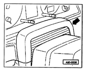
• Tilt upper cover forward an remove upward.
