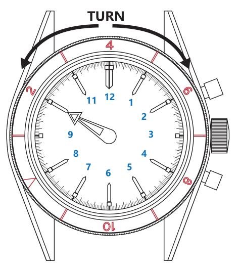
The Gemini's bezel rotates in both directions.
