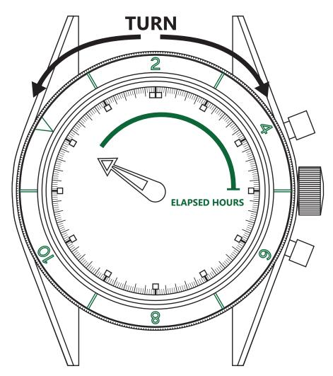
The Gemini's bezel rotates in both directions.
