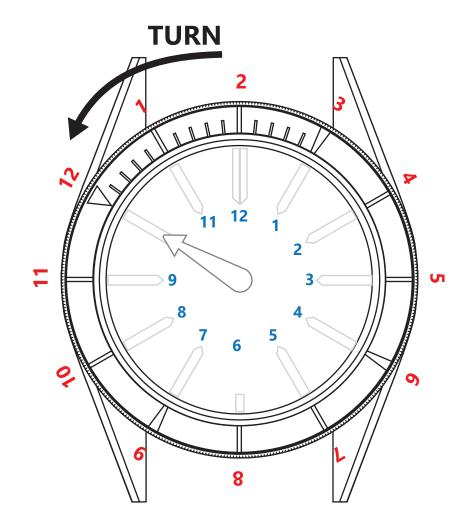
The timing bezel rotates counter-clockwise.
