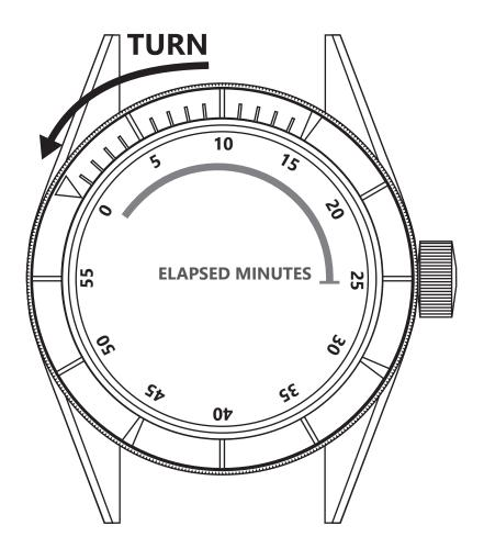
The timing bezel rotates counter-clockwise. Simply turn the bezel triangle to the current position of the minute hand in order to show elapsed time.
