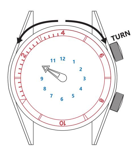
The Hydra's internal bezel rotates in both directions via the crown at 2 o'clock.
