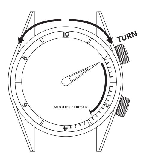
The Hydra's internal bezel can also track minutes elapsed. Using the crown at 2 o'clock, simply turn the bezel triangle to the current position of the minute hand in order to show elapsed time moving forward.
