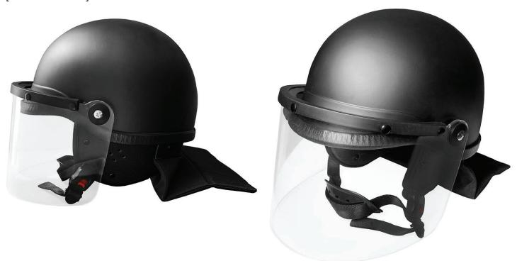
The New Damascus® Riot Control Helmet features a high-impact, ABS molded shell with neck protector and clear/polycarbonate tactical face shield that is gasket sealed. The helmet straps on with a quick-release retention system with chin cup. Provides full head and face protection against almost all NON-ballistic threats, such as chemicals, rocks, bottles and other projectiles.
