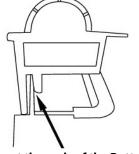
Insert the ends of the Bottom Panel found underneath the Right Panel into the groove of the Wheel Frame.
