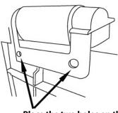
Place the two holes on the Wheel Frame over the plugs underneath the Bottom Panel.
