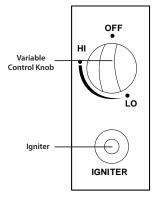
When lit for the first time the heater may emit a slight odor and smoke. This is a normal and temporary condition. Emitter screen will become a bright red due to the heat. The color is more visible at night. Flame patterns should be a blue flame; these flames should not be yellow in color; indicating an obstruction of airflow through the burners.
