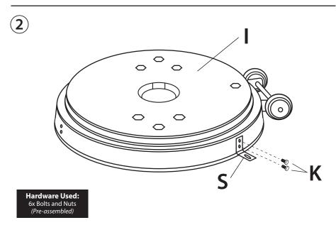
Insert two M6x10 Bolts (K) through the two eyelets of an Anchoring Arm (S), through a set of eyelets found on the side of the Base (I), and tighten down using two M6 Nuts (L). Follow this step to assemble the remaining two Anchoring Arms (S) to the Base (I).
