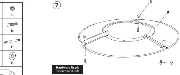
Note: Remove the protective film from the three Reflector Panels (A) before proceeding further. Slide two Reflector Panels (A) together and insert one Small Screw (V) through the panels [underneath] along the outer rim and use one Cap Nut (U) to hold the parts together. Follow this step to assemble the remaining Reflector Panel (A) to the two previously assembled. Note: Do not tighten Cap Nuts (U) down until Step 8 has been completed.
