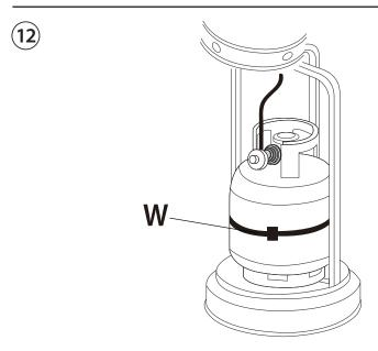
Lift the Tank Housing (E) up and place your 20lbs LP cylinder tank in the center of the Base (I). Use the Strap (W) to hold the tank in place.
