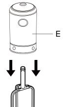
Place the Tank Housing (E) over the previously assembled parts so that it rests upon the Base (I).
