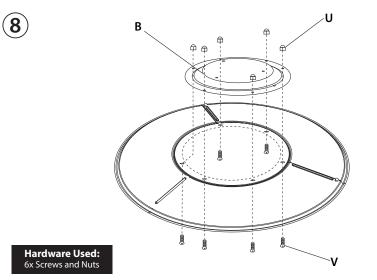
Note: Remove the protective film from the Center Reflector (B). Place Center Reflector (B) on top of the previously assembled Reflector Panels (A). Insert six Small Screws (V) through the inner rim of the Reflector Panels (A) [underneath], through the eyelets on the outer rim of the Center Reflector (B), use six Cap Nuts (U) to hold the parts together. Once all parts are assembled, tighten all Cap Nuts (U).
