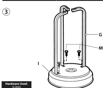
Insert one M8 Bolt (M) through the bottom Support Leg (G) and into the top of Base (I). Follow this step to assemble the remaining two Support Legs (G) to the Base (I).
