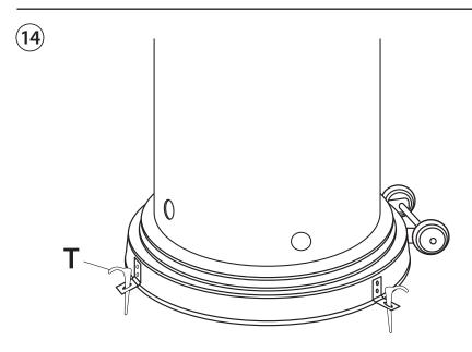
Use a hammer to drive the three Stakes (T) through Anchoring Arms (S), and into the ground to hold the Patio Heater in place.
