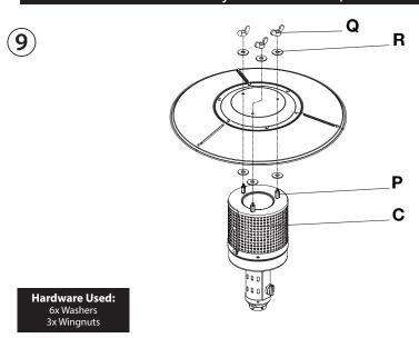
Place three Washers (R) through the top-ends of the Studs (P). Place the assembled reflector through the top-end of studs, use another three Washers (R), and screw down three Wingnuts (Q) to hold reflector in place.
