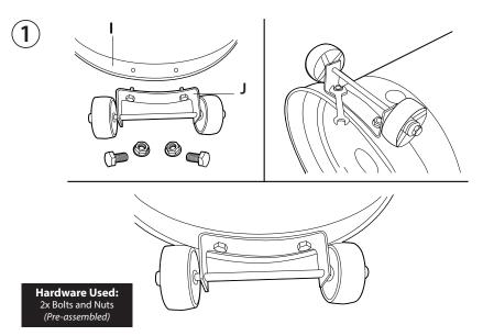
Place the base of the Wheel Assembly so that it is flush with the side of the Base (I). Insert two M6x10 Bolts (K) through the Wheel Assembly (J), through the Base (I), and tighten down using two M6 Nuts (L).
