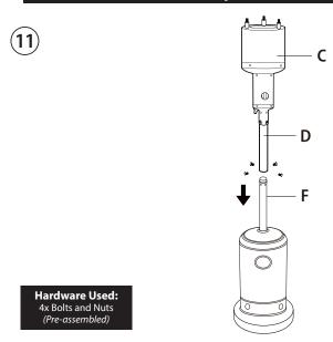
Unscrew the four Bolts that are preassembled near the top of Post Support (F). Insert Regulator (H) through Post Support (F). Insert Post (D) over the end of Post Support (F). Tighten down the Bolts through the bottom of Post (D) and back into the top of Post Support (F).
