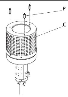
Screw down one end of the three Studs (P) into the top of the Head Assembly (C).
