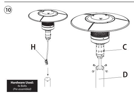
Unscrew the four Bolts that are preassembled near the bottom of the Head Assembly (C). Insert the Regulator (H) through Post (D). Tighten down the Bolts through the top of Post (D) and back into the Head Assembly (C).
