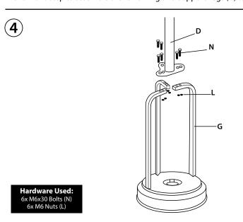
Place Post (D) on top of the three Support Legs (G). Insert two M6x30 Bolts (N) through the base of Post (D), through the top of Support Legs (G), and tighten down using two M6 Nuts (L). Follow this step to assemble Post (D) to the two remaining Support Legs (G).
