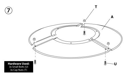
Note: Remove the protective film from the three Reflector Panels (A) before proceeding further. Slide two Reflector Panels (A) together and insert one Small Bolt (U) through the panels [underneath] along the outer rim and use one Cap Nut (T) to hold the parts together. Follow this step to assemble the remaining Reflector Panel (A) to the two previously assembled. Note: Do not tighten Cap Nuts (T) down until Step 8 has been completed.
