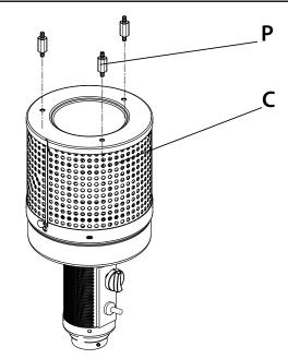
Screw down one end of the three Studs (P) into the top of the Head Assembly (C).
