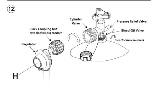
Turn the valve on the LP cylinder tank clockwise to close the propane tank. Attach the Regulator (H) to the LP cylinder tank by turning the coupling nut clockwise. Ensure that the connection is tight and secure.
