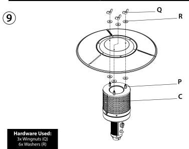
Place three Washers (R) through the top-ends of the Studs (P). Place the assembled reflector through the top-end of studs, use another three Washers (R), and screw down three Wingnuts (Q) to hold reflector in place.
