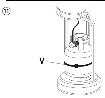
Lift the Tank Housing (E) up and place your 20lbs LP cylinder tank in the center of the Base (I). Use the Strap (V) to hold the tank in place.
