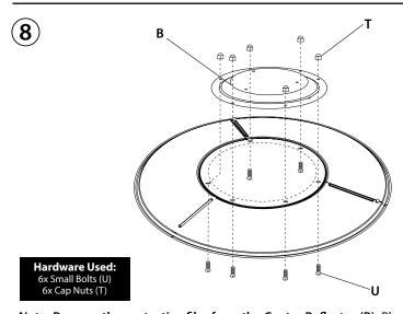
**Note:** Remove the protective film from the Center Reflector (B). Place Center Reflector (B) on top of the previously assembled Reflector Panels (A). Insert six Small Bolts (U) through the inner rim of the Reflector Panels (A) [underneath], through the eyelets on the outer rim of the Center Reflector (B), use six Cap Nuts (T) to hold the parts together. Once all parts are assembled, tighten all Cap Nuts (T).
