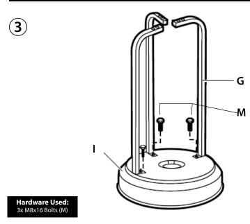
Insert one M8x16 Bolt (M) through the bottom Support Leg (G) and into the top of Base (I). Follow this step to assemble the remaining two Support Legs (G) to the Base (I).
