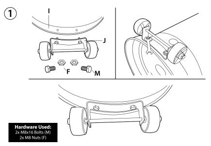
Place the base of the Wheel Assembly (J) so that it is flush with the side of the Base (I). Insert two M8x16 Bolts (M) through the Wheel Assembly (J), through the Base (I), and tighten down using two M8 Nuts (F).
