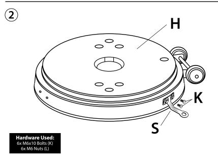
Insert two M6x10 Bolts (K) through the two eyelets of an Anchoring Arm (S), through a set of eyelets found on the side of the Base (I), and tighten down using two M6 Nuts (L). Follow this step to assemble the remaining two Anchoring Arms (S) to the Base (I).
