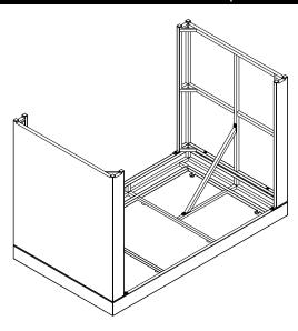
**Step 3:** Tighten all bolts left loose throughout assembly process.
