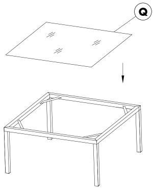
Turn the assembled table to its upright position and place the Table Glass (Q) onto the Table Rim (P).
