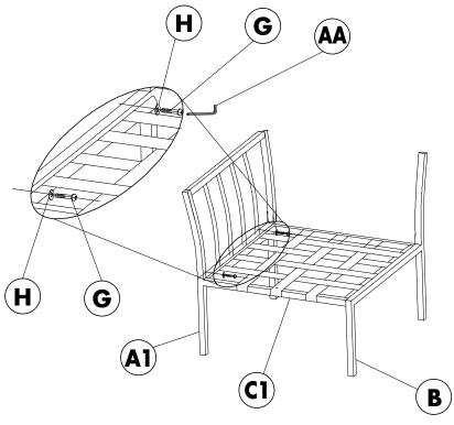
Attach the Seat (C1) to the Right Leg (A1) using Screw (G) and Washer (H).
