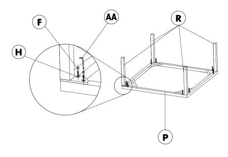
Place Table Rim (P) upside down on a clean flat surface. Screw the Table Legs (R) to the corner of the Table Rim (P) using Screw (F) and Washer (H).
