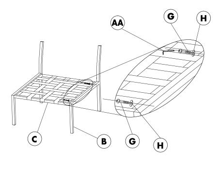
Attach Seat (C) to Left Leg (A) using Screw (G) and Washer (H).
