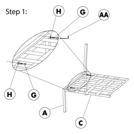
Attach Seat (C) to Right Leg (A) using Screw (G) and Washer (H).
