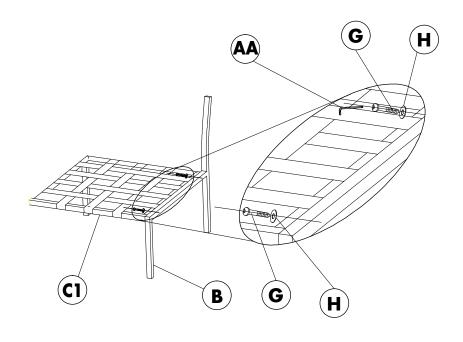
Attach Left Leg (B) to Seat (C1) using Screw (G) and Washer (H).
