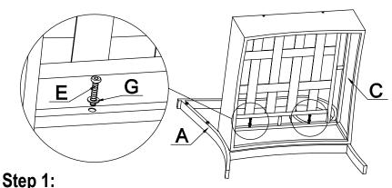
Set Armrest (A) on the ground so that the rear leg is to your left and front leg is to your right. Set Chair Seat (C) onto Armrest (A) as illustrated here. Insert two Bolts M6x30 (E) with Washers (G) through interior frame bar of Chair Seat (C) and into the screw-threading found on the middle horizontal bar of Armrest (A); do not tighten bolts all the way until assembly is completed.
