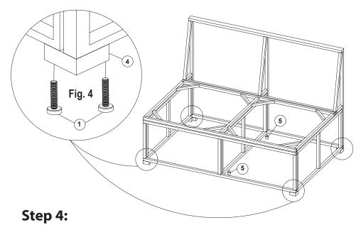
Turn the sofa upside down. Place Corner Feet (4) at either corner of sofa bottom. Insert two M6x25 Bolts (8) through each Corner Foot (4) and into bolt-threading found at the bottoms of all previously assembled parts; see Figure 4. Tighten bolts left loose throughout assembly process using Hex Key (7). Screw in two Feet (5) into bolt-threading on the bottom Support Panel (B5). Turn the sofa right-side up when finished.
