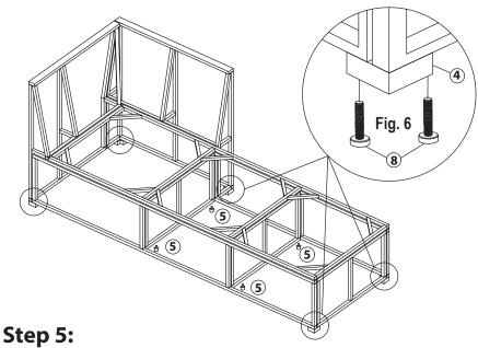
Turn the chaise upside down. Place Corner Feet (4) at all corners illustrated above. Insert two M6x25 Bolts (8) through each Corner Foot (4) and into bolt-threading found at the bottoms of all previously assembled parts; see Figure 6. Tighten bolts left loose throughout assembly process using Hex Key (7). Screw in two Feet (5) into bolt-threading on the bottoms of both Supports (C7). Turn the chaise right-side up when finished.
