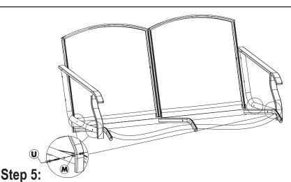
Place the bottom of Armrest (D) against the end of Swing Seat (H). Insert one Bolt M6x60 (U) through the bottom-front of Armrest (D), through Spacer (M), and through the hole found at the front-side of Swing Seat (H). Tighten a nut halfway down on bolt to hold parts in place with Wrench and Hex Key (X). Follow these steps to assemble the second Armrest (D) to the opposite side of Swing Seat (H).
