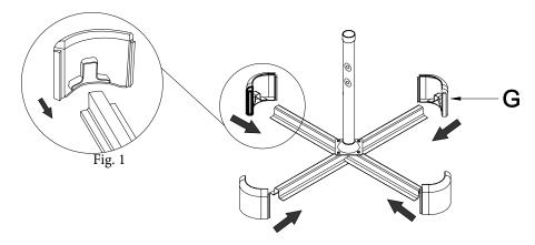
Step 3: Insert Frame Corners (G) to the ends of Bottom Cross Bar (A) and Top Cross Bar (B); see Fig. 1.
