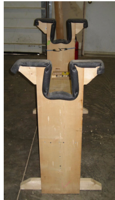
FIGURE C-7. (above and left) Shaping stand of 2x12 lumber.
