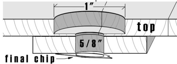
**FIGURE 2-26.** Holes for the vent that will allow flush-mounting. Surface-mount would have only a 5/8" hole and no backing pad
