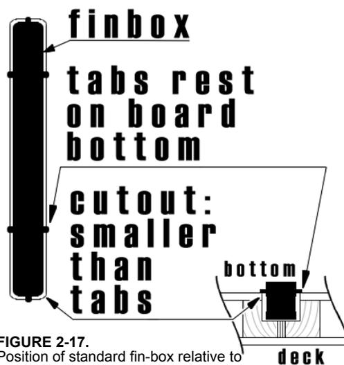
**FIGURE 2-17.** Position of standard fin-box relative to mortise, viewed from bottom and in cross-section.
