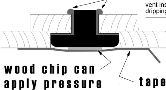
**FIGURE 2-27.** Inverting the board after vent installation keeps epoxy from dripping out into the board's interior.
