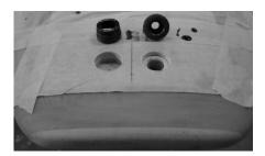
This task will cause the vent to be either flush- or surface-mounted, and a leash cup will be installed. These are visually strong elements, so we will want them symmetrically installed, a decision which was made in Step 7.2 when the blocking was installed.
