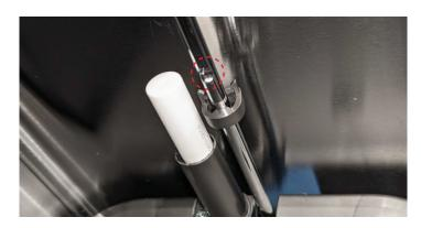
3. Clip pusher from rod. Make sure the rod protrusion is within pusher gap.
