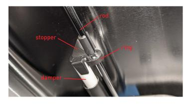
3. Using flathead screwdriver, push ring piece to disengage it from pusher.
