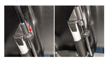
4. Remove (unclip) pusher from rod.
