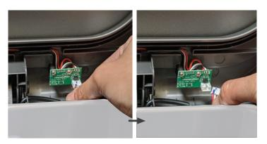
8. Use screwdriver to slide tabs toward the center. Make sure both tabs have been moved to their end-most positions.
