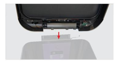
2. Slide tabs outward using screwdriver. Start with the left side first. **Tip:** You may need to constantly adjust lid while sliding the right tab.
