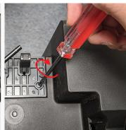
4. Insert rod into new pedal. Connect rod and pedal to air damper. Push rod back into its groove.
