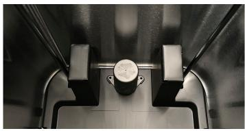
2. Place new air damper into can. **Tip**: Ensure screw holes
