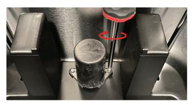
4. Insert piston screw and bracket into their respective slot. Tighten piston screw using screwdriver.
