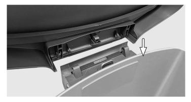
3. Firmly press on each pin until it snaps. This means they are now locked into place.
