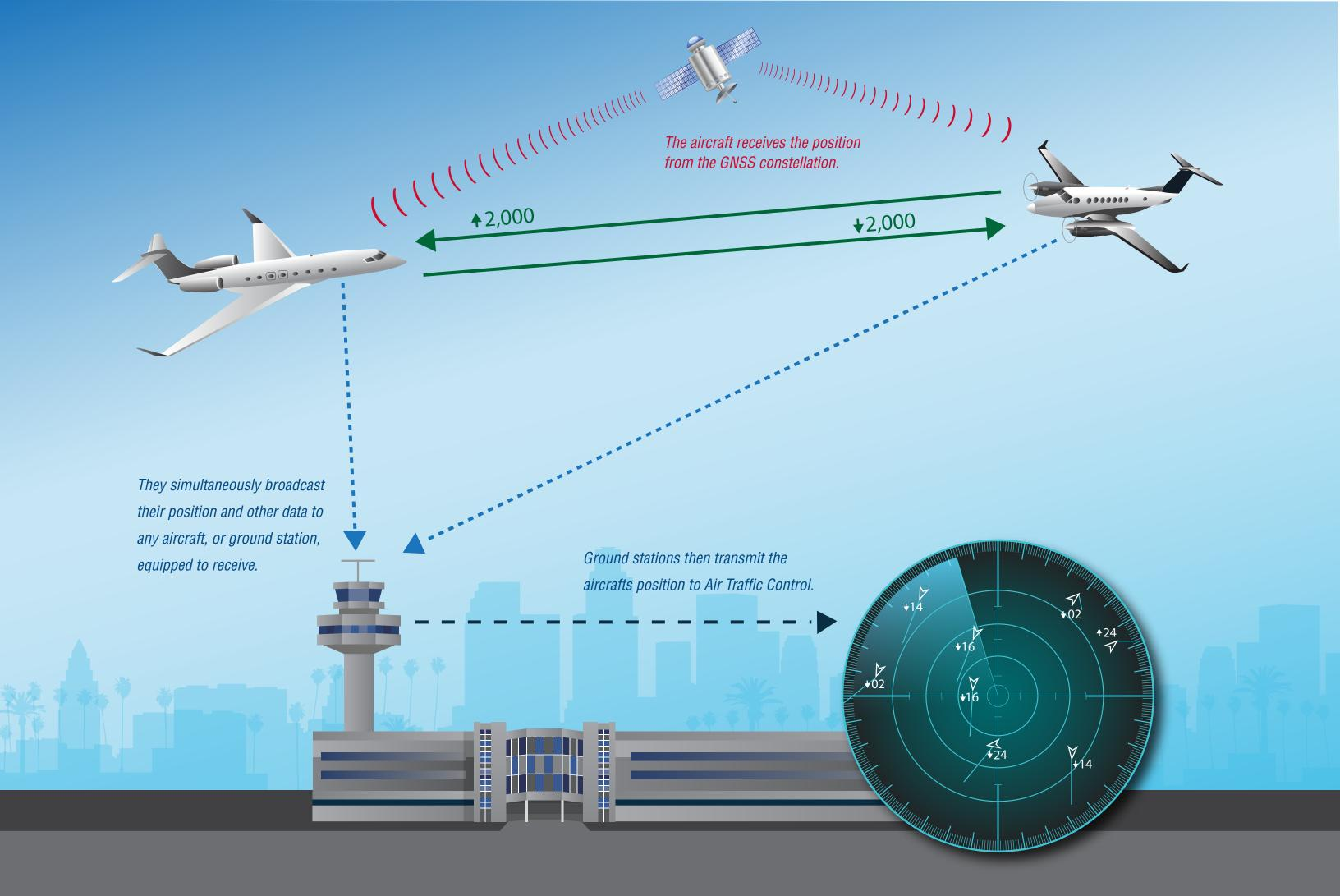
Improved Safety - ADS-B provides flight crews and controllers a more accurate traffic picture which is expected to reduce the number of mid-air collisions as well as reduce airport surface incidents and accidents.
