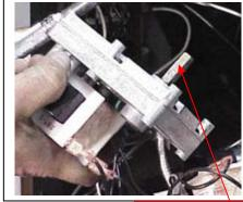
one of the remaining bolts, then check the auger for smoothness again; if free, tighten the last bolt.
