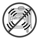
Overfiring the appliance may cause a house fire. If a unit or chimney connector glows, you are overfiring.
