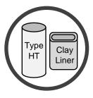
This appliance must be connected to a listed high temperature (UL 103 HT) residential type chimney or an approved masonry chimney with a standard clay tile, or stainless steel liner.
