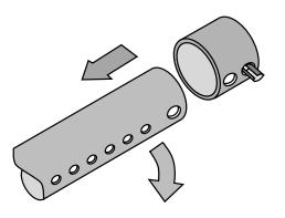
**b** Slide the air tube to the left, swing it down and remove from the firebox.
