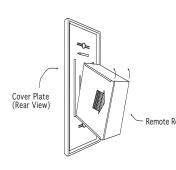
Position the receiver as shown in diagram to the left with lower tab on cover plate inserted into groove of receiver (Make sure LEARN hole on cover plate properly aligns with remote receiver). Pull receiver up and snap into top tab of cover plate.
