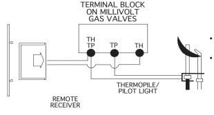
Connect one wire from the remote receiver to the TH terminal on the gas
