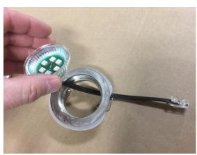
Insert one of the LED bulbs into the front of the housing and screw the lens assembly back in place to secure the bulb.
