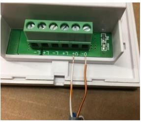
Strip about 3/16" insulation from each wire before inserting into the terminal block.
