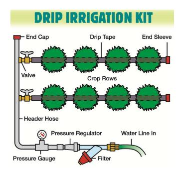
A well-designed drip irrigation system benefits the environment (and your plants!) by conserving water and fertilizer, and requires very little labor. Drip irrigation sends a uniform distribution of water directly to the root zone of plants, avoiding waste and runoff. A system such as ours tends to use up to 50% less water than conventional systems, and minimizes such negatives as soil compaction, erosion and weed growth. Its use also tends to minimize leaf burn, and fungal diseases.
