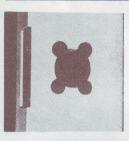
Drill four holes 10mm dia. (3") through the door. Drill one hole 32mm dia.  $(1\frac{1}{4}")$ through the door. Chisel a 2.5mm  $(\frac{3}{32}")$  deep recess in the edge of the door to house the lock forend and countersink the holes 8mm  $(\frac{5}{16}")$  dia. to clear the countersinks on the lock forend.
