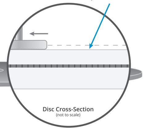
When sufficient repair time has passed, the disc will look and play like new again. The material removed is usually less than 1% of the disc's thickness, allowing for future repairs.
