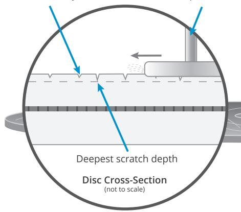
The disc polishing process takes layers off the shiny side of the disc, this is carried out until the depth of the deepest scratch has been reached. Then the surface will be scratch free.
