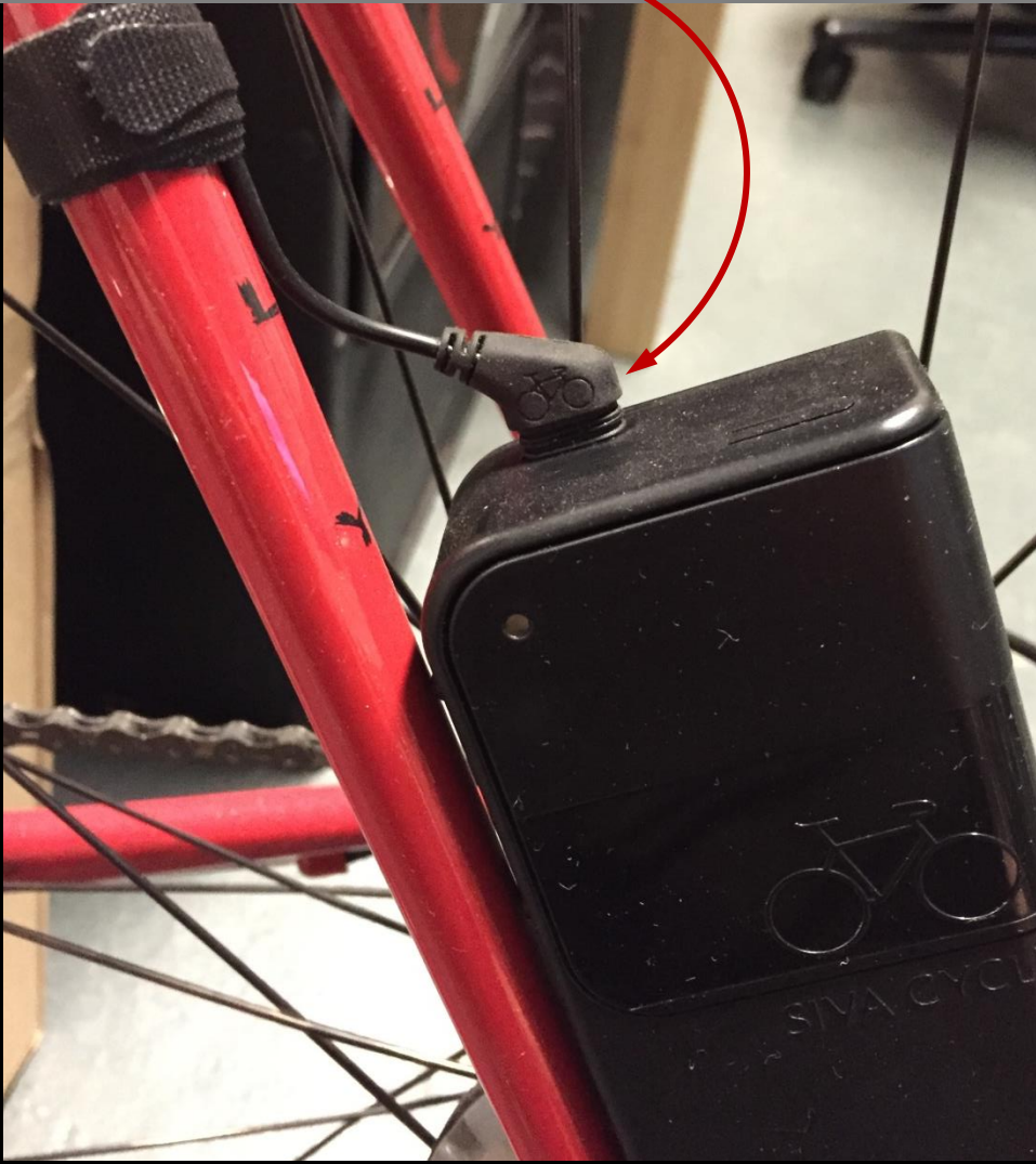
Incorrect: Not fully seated
