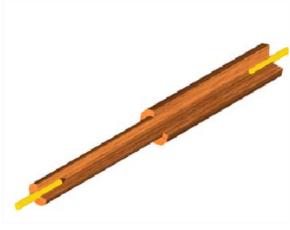
1/4 SECTION REMOVED TO SHOW 3/32" PIN RECESS
