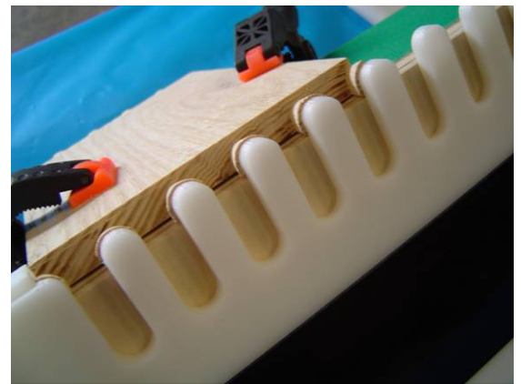
Inspect cut before removing from template guide. Assure all cuts are complete.
