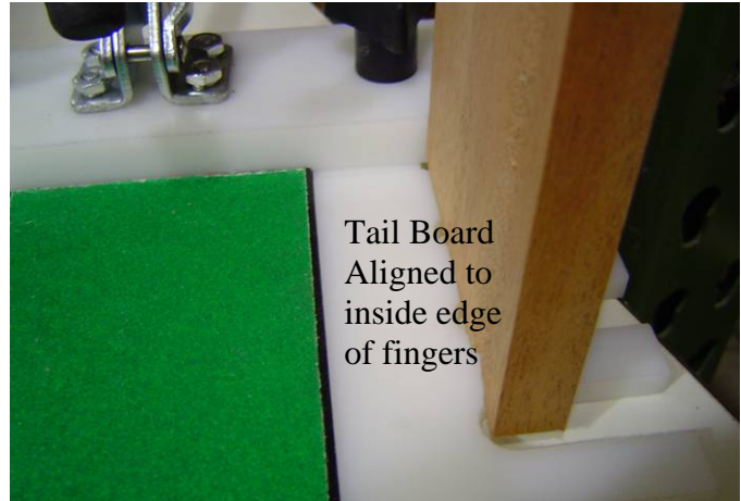
Use tail board as set gauge against inside edge of pin template.
