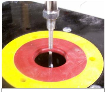
Figure 1 Guide pin aligned with bit
