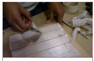
Figure 4 Use heavy duty double stick tape
