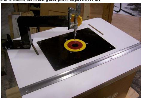
Figure 2 Pin router can be bolted or clamped to any table
