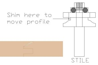
If the bit spins on the shaft recheck for fit and shim as necessary before proceeding.
