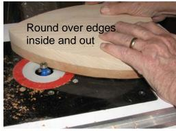
Select a bit no larger than half the width of the wall thickness. Sand inside and outside to remove any tool marks.
