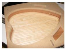
Make a final pass with a light cut and inspect to be sure that all tooling marks are removed and all details are exposed.
