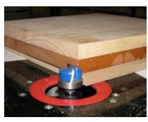
Set bit height. Invert over router table and carefully use multiple passes and clear chips frequently until all tooling marks from drilling operation are removed.
