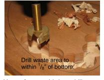
Use a forstner bit in a drill press at low speed only (<600 RMP).
