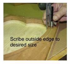
Reference lines are provided as a guide to allow approximately ½" thick walls, but you may make the outline any shape or thickness.
