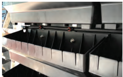
6) Installation of auto-irrigation pipes and emitters.
