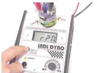
This is the rpm screen (x100 units)
