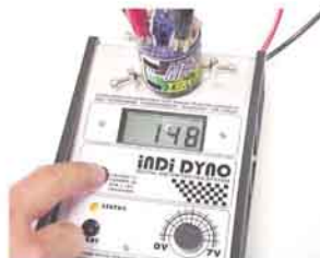
This motor is running at 14,800rpm
