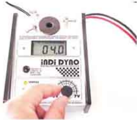
Adjust the voltage output to 4.0
