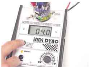
Adjust voltage output to 4.0 again
