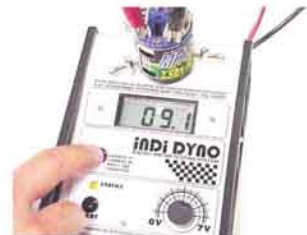
This motor draws 9.1 Amps during test
