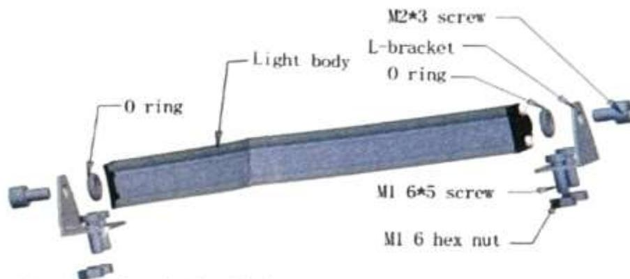
Note: For L bracket installation, O rings must be added on both sides.
