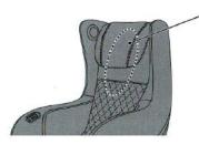
Inspected area: The fabric of traveling sections of the massage wheels on the backrest
