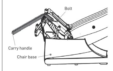
Attach carry handle as shown; slide bolt through carry handle and into frame.
