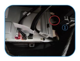
8. Find the second gray plug of the host above the passenger's footwell and connect it to plug 1
