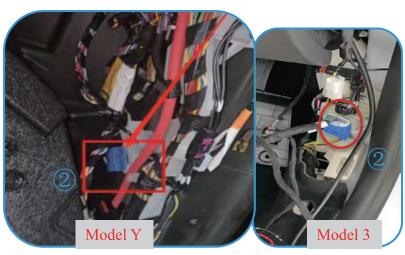
9. Connect the plug ② to the blue plug under the A pillar of the front right seat
