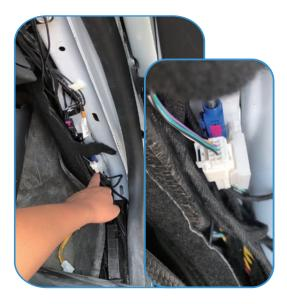
8. Connect the plug ③ to the white plug under the A pillar of the front right seat
