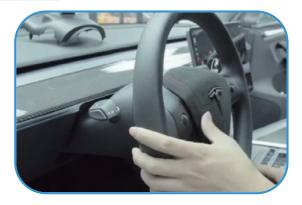
1. Slide the steering wheel to the bottom and then turn left to move the steering wheel to the the outermost position
