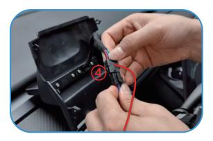
3. Then pry the harness plug 4 from the upper cover plate of the driver's footwell and pull the harness to the upper part according to the instructions in the picture and plug it into the screen
