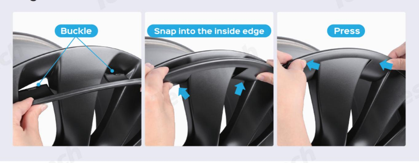
Align the next hub protector segment with the edge of the previous one and press it in. Repeat this step for all segments.
