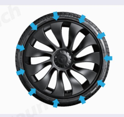
Blease check again if the hub protector fully covers the wheel rim edge, attempt to pry the hub protector outward with your hand, if it comes off, press firmly to ensure it is properly installed. (To avoid fall off during drive).
