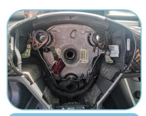
8. Then pull out the steering wheel. If the steering wheel is too tight, shake it left and right and pull it out slowly.
