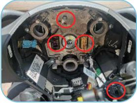
10. Then remove the harness of the original steering wheel and install it on the new steering wheel, then buckle the speaker harness and plug in the plug.
