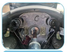
7. Screw out the steering wheel screw with a large H10 wrench.
