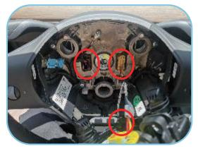
5. Take out the airbag and pull out the airbag plug and steering wheel plug. then take off the airbag
