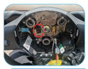
6. Note that the steering wheel plug must be pulled out to avoid pulling out the hairspring.
