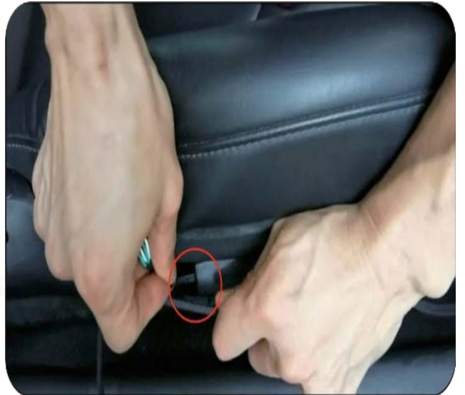
16. Connect the seat adjustment harness and route the harness from the back of the seat
