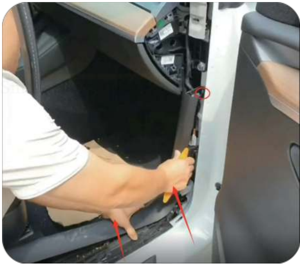
3. Remove this clip and take out the kick guard trim panel
