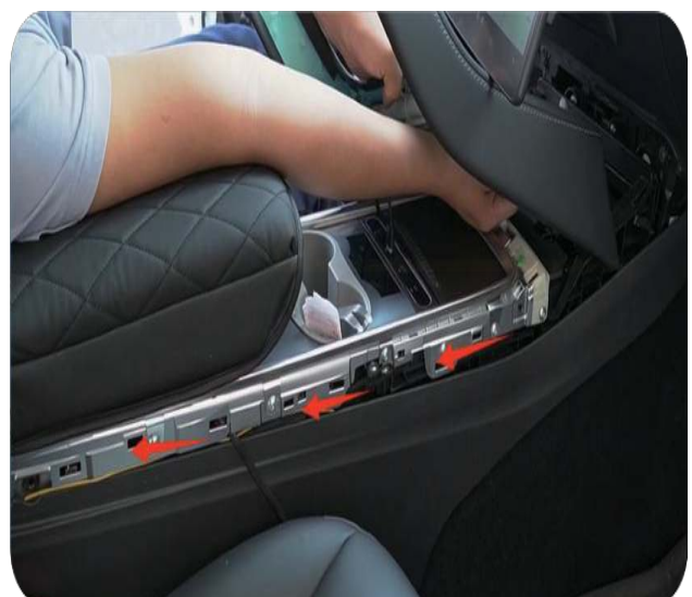
12. Run the power wire from the center console side position towards the rear
