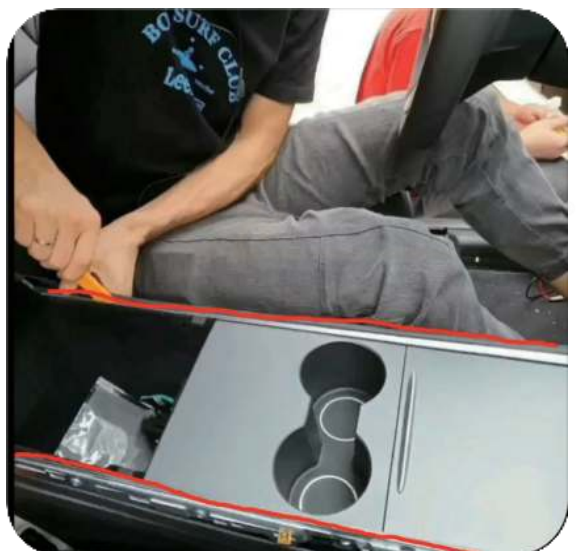
6. Use a pry bar to open the center console side trim panel
