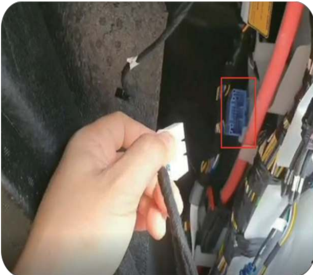
9. Connect the protocol cable to the blue plug on the right side of the passenger seat
