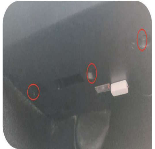
4. Remove the passenger side lower cover (left side clip, right side screw)
