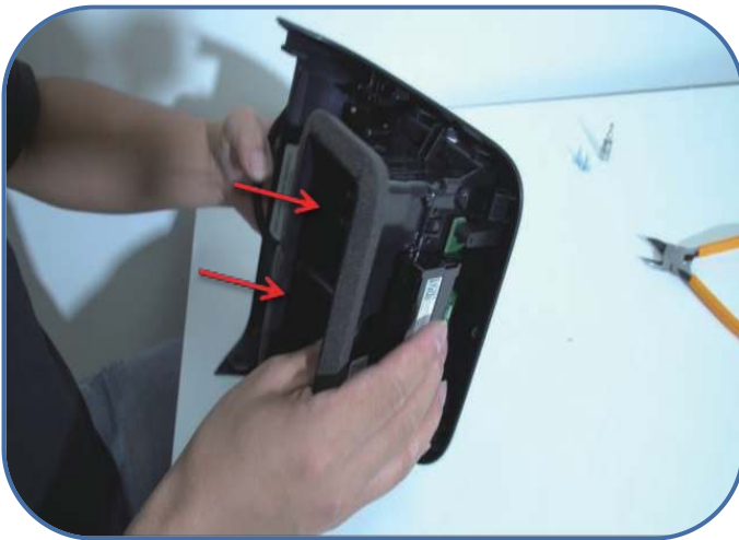
9. Screw on the screws on the upper part of the A/C outlet
