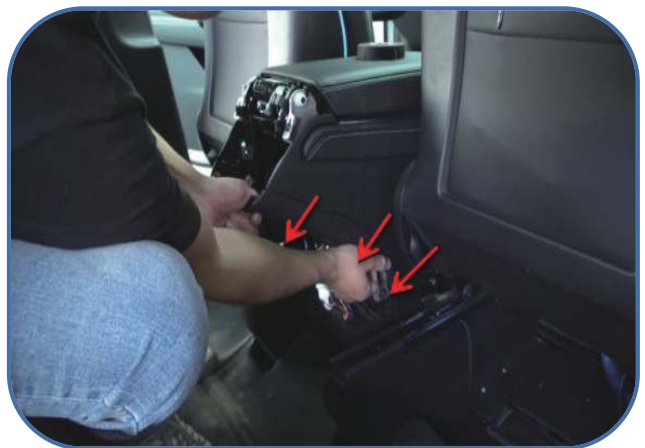
12. Pry the cover plate behind the central armrest saddle in the direction of the arrow
