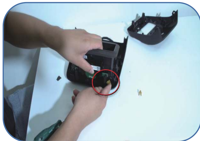
11. Install the clips onto the screen panel
