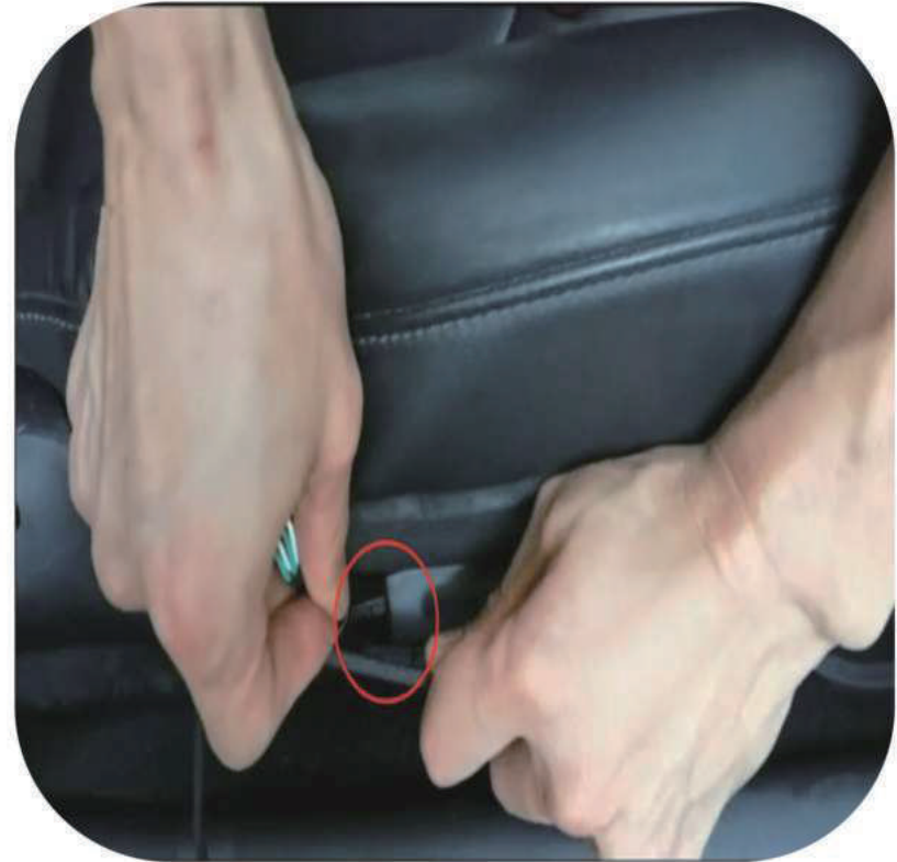
16. Connect the seat adjustment harness and route the harness from the back of the seat
