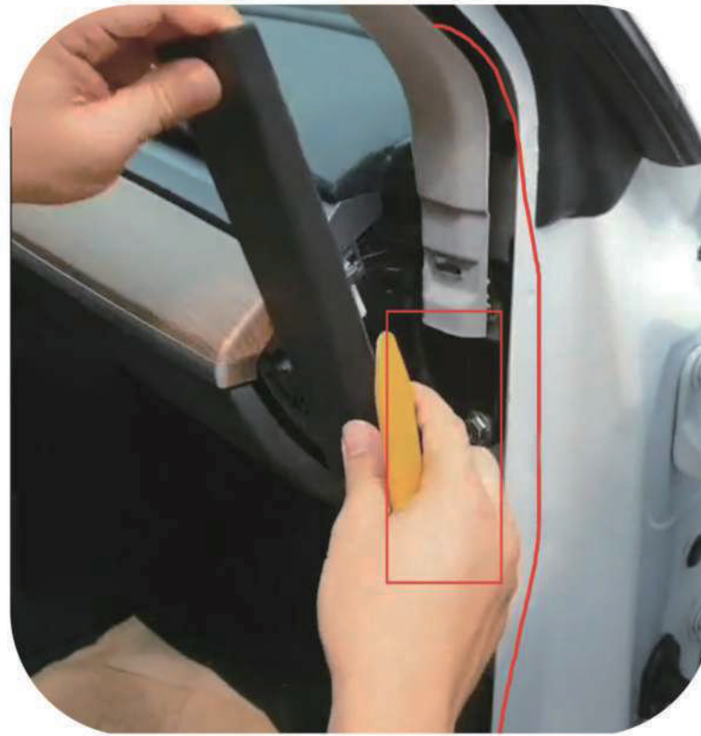
2. Pull open the strip and remove this trim panel
