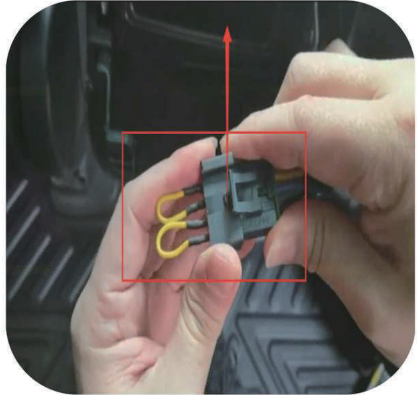
14. After plugging in the dedicated plug for the Model Y, insert it into the air vent
