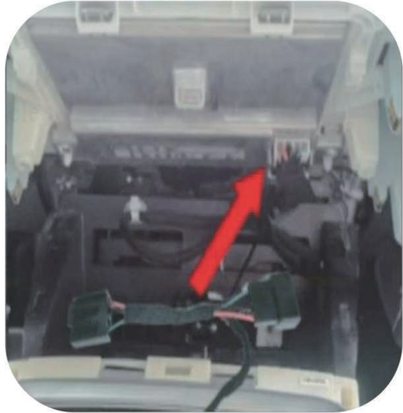
8. Connect the power cable adapter to the wireless charging plug
