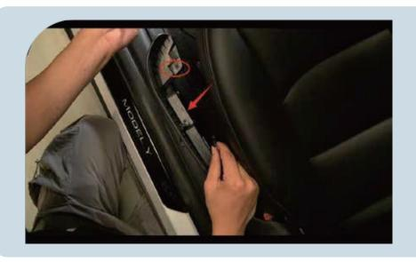
22. Remove the screws of the seat adjustment panel, detach the panel, and unplug the seat adjustment connector
