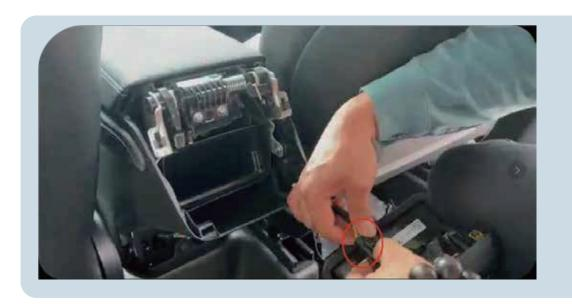
5. Unplug the power cable of the rear air conditioning
