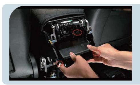
12. First, snap the two clips on the bottom into place, and then tighten one screw on the top to secure it
