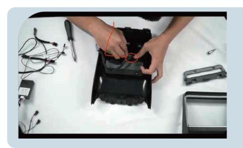
11. Connect the screen adapter cable properly and route it along this path (There is a locking pin. Please be careful when inserting the cable)
