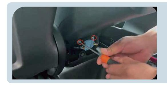
3. Remove these two screws to take out the air vent baffle
