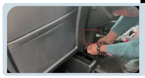
2. Use a pry bar to remove the lower panel of the rear air vent
