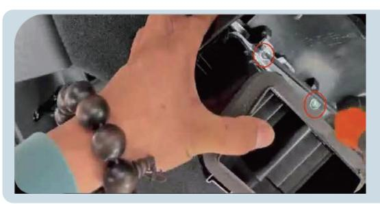
6. Remove the two screws of the rear air conditioning vent
