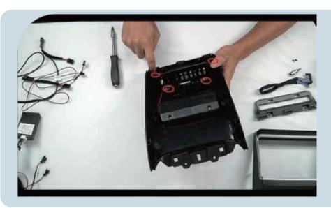
10. First, align the charging module in position and screw in the screws partially. Then, tighten the remaining screws to secure it in place
