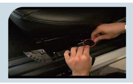
23. Connect the seat adjustment wire from the original car to the driver's seat adapter cable, same operation to the passenger seat
