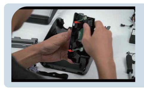
9. Assemble the removed charging module onto the corresponding mold
