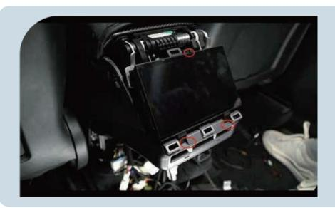
18. Tighten these three screws to secure it in place
