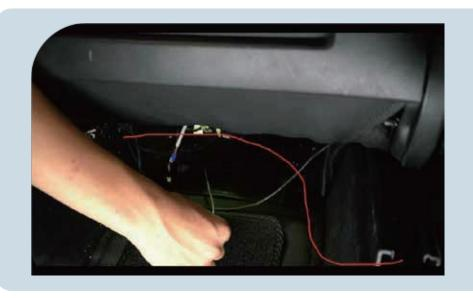
21. Route the driver's seat adjustment wire along the seat position (Make sure to hide the wire properly)
