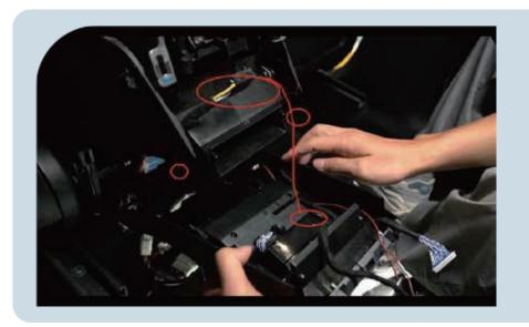
15. Insert the plug into the socket indicated in the connection diagram, aligning it with the corresponding holes, and secure it (Be sure to fasten it tightly)
