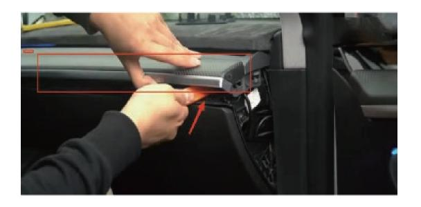
1. Use a pry bar to pry open the left and right small side panels.
