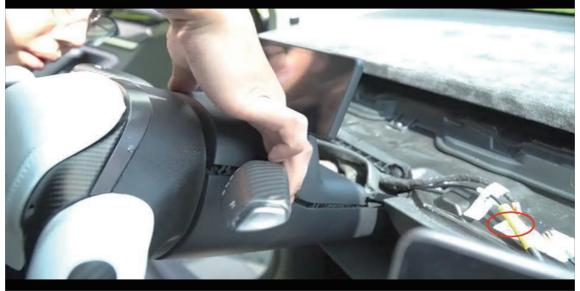
9. Once the fish tape is visible from the passenger side, pull it inside
